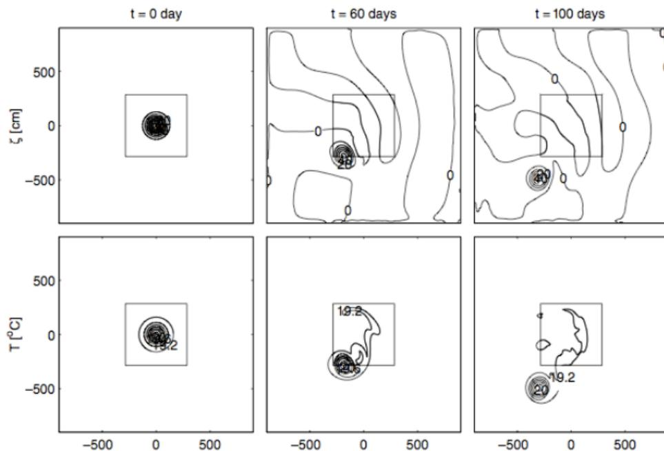
Fig. 1. Reference solution (V1) for the baroclinic vortex for days 0, 60 and 100. Top: sea surface elevation [cm], the contour interval is 10 cm. Bottom: sea surface temperature [°C], the contour interval is 0.2 °C. The box represents the embedded domain, in this case using the same resolution as the parent grid (10 km).
