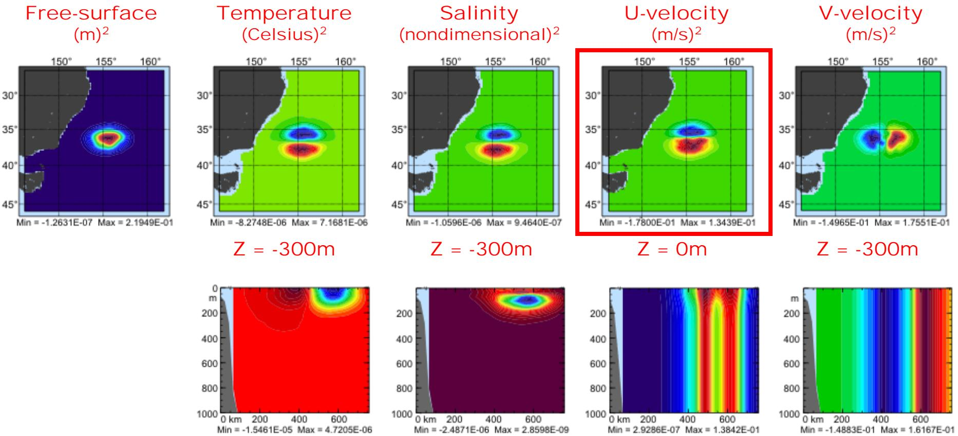
The cross-covariances are computed from a single **U-velocity** observation at the surface using multivariate physical balance relationships.
