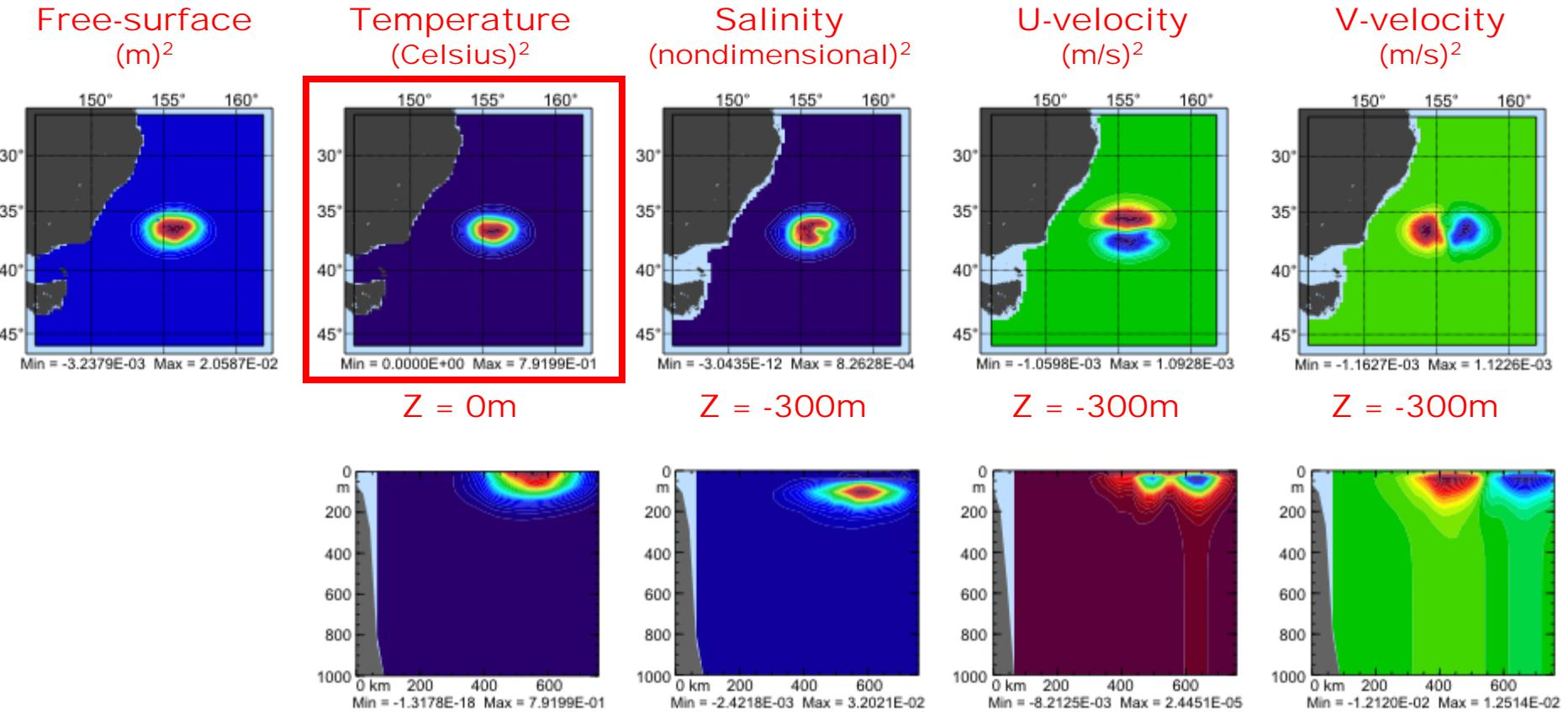
The cross-covariances are computed from a single **temperature** observation at the surface using multivariate physical balance relationships.
